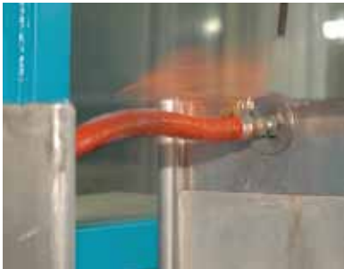
Techflex silicone jacketed fiberglass is tested under pressure to destruction to insure reliable fire protection for your fuel and hydraulic lines.
